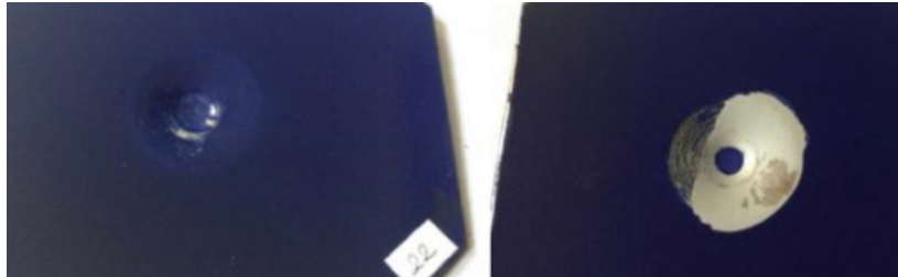
Figure4; Impact test results showing – good adhesion - Poor adhesion
