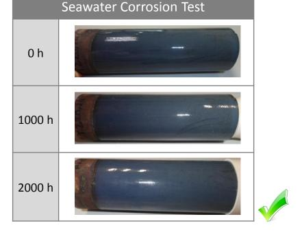
High corrosion resistance for offshore applications
