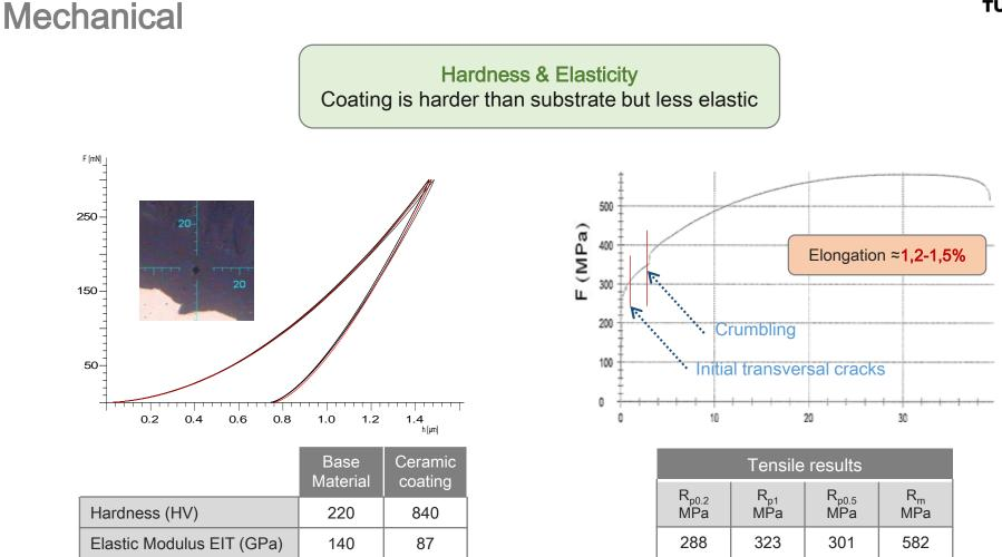
Hardness and elasticity properties can be improved by modifying structure and composition of ceramic compounds and process conditions
