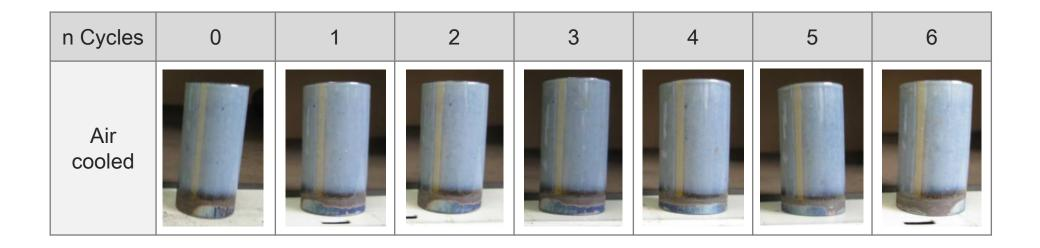
Different working temperature and thermal cycling resistance can be achieved by modifying structure and composition of ceramic compounds
