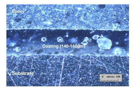
Typical coating thickness range: 100-200 µm
