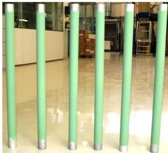
Figure 1. Tubes with RT-100 ceramic coating in green (biscuit) state
