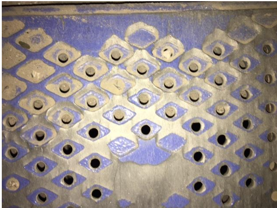
FAQ-4: The central spot was without coating since the beginning.
