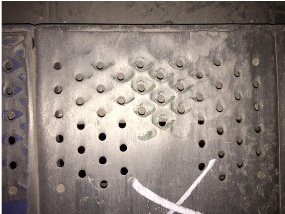
Plate coated with K-100: just some traces in the most refrigerated areas, close to the wind holes.
