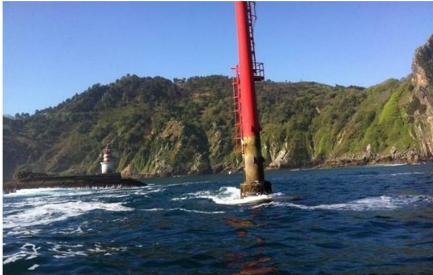
Figure 3. Test rig for antifouling tests (samples attached to the splash / tidal part) developed by Kera-Coat/IK4-Cidetec).
