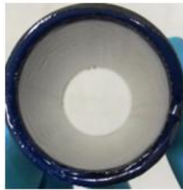
Figure 2. Carbon Steel tubes coated with ceramic coating
