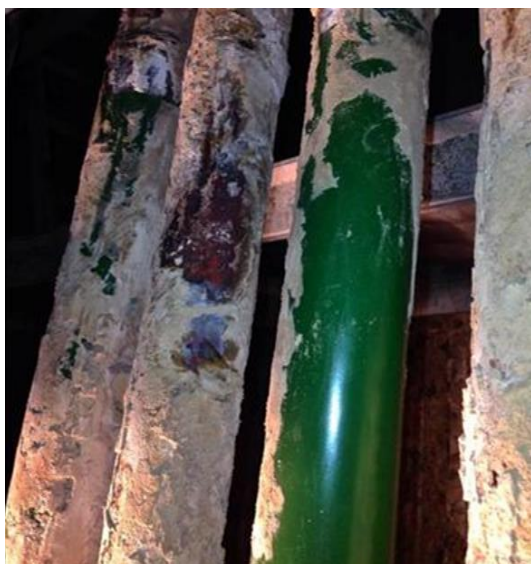
Figure 11: Tubes after 1 year and after three years before and after cleaning the ash by hand with a glove
