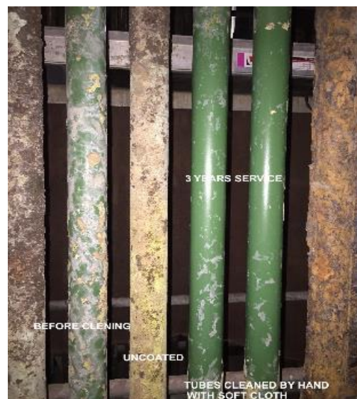
Figure 11: Tubes after 1 year and after three years before and after cleaning the ash by hand with a glove
