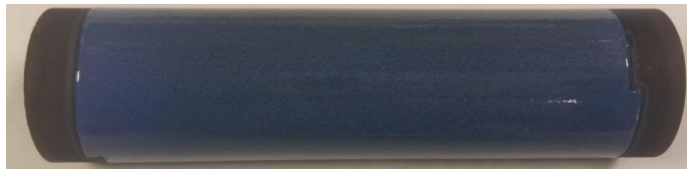
Figure 6 : Water quenched from 850°C to 20°C.
