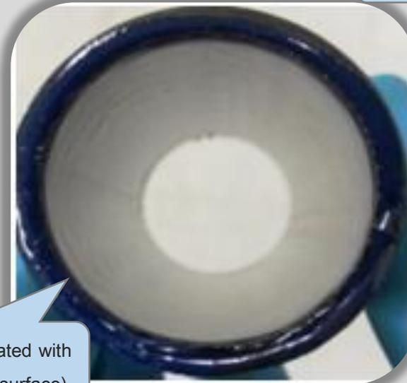
Carbon steel tubes coated with ceramic coating (inner surface)
