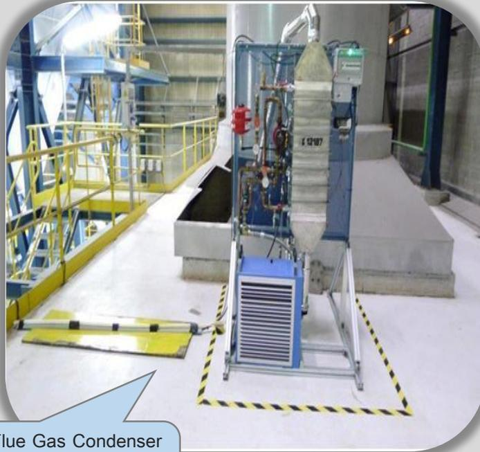
5KW Cold End Flue Gas Condenser prototype at a Waste to Energy Plant (SPAIN)
